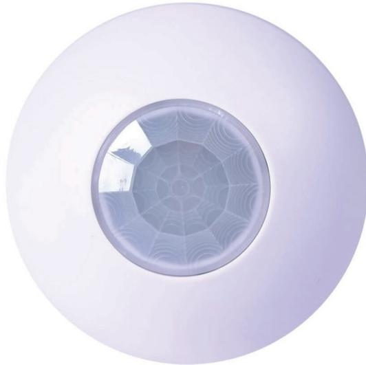
The multi functional sensor Motion 360 KNX is suitable for ceiling mount. It monitors movement, brightness and temperature with a detection angle of 360°. The Motion 360 KNX comes with two dry contacts and several logic functions.
